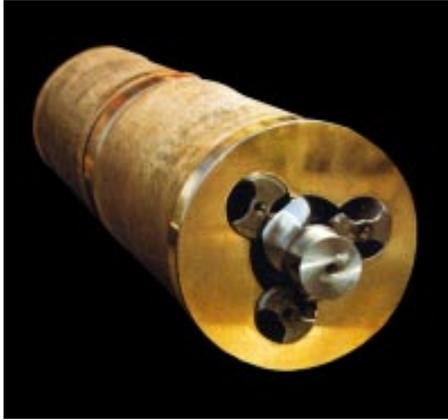
Incorporating a third idler rotor in the Imo design (one power rotor and three idler rotors) automatically creates a complex internal leakage path, providing a restricted interconnection among cavities. Pressure rise therefore is more constant and gradual. Bubble implosion is less abrupt
