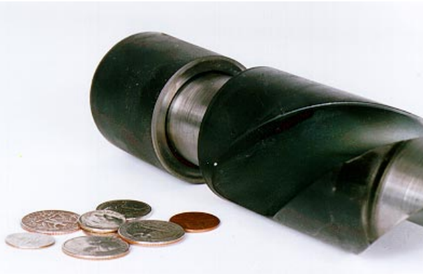
Figure 10 Running Clearance Increase Caused By Very Fine Contaminant
