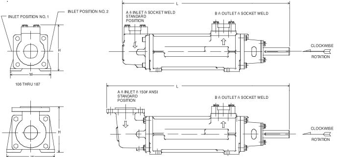
Picture depicts iron-cased pumps. For steel-cased pump dimensions contact the factory
