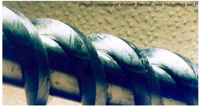
Figure 9 Pump Rotor Damage Caused By Hard Contaminant
