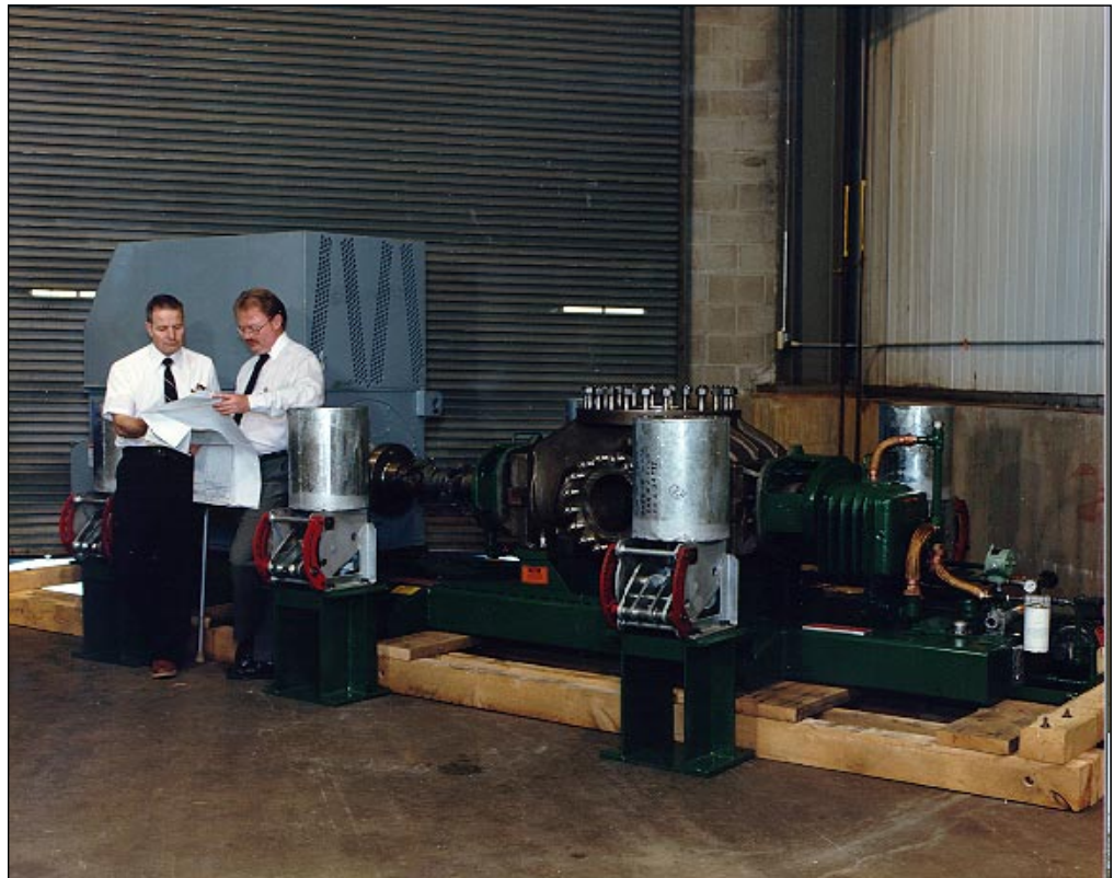
Figure 6 Final Inspection of Stainless Steel Adhesive Process Pump with Thermal Compensation Mounts
